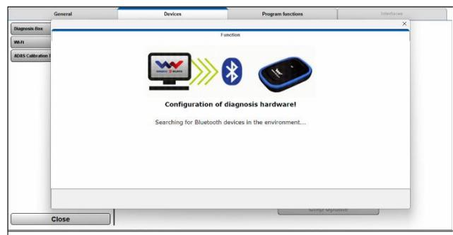
→ The Bluetooth connection to the W.EASY CONNECT should now be displayed and identified as "W.EASY CONNECT + BT\_Serial number", as shown in the following illustration.
